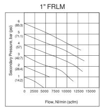
Flow graphs are for 40µm filterations only
