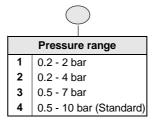
Ordering example: Filter Regulator Combination and Lubricator Modular - 3/8 size ( with G3/8 port ) with 5µm Filter and pressure range 0.5 - 7 bar: Ordering No: FRCLM 146213.
